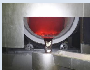
Pouring Molten Aluminum Notice the mouth design that keeps slag Away from the pour area.
